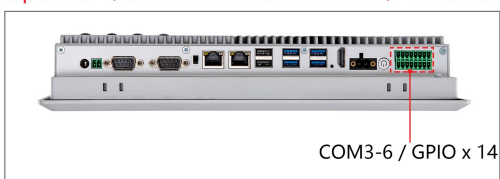
Optional I/O View : iDOOR-4x COM / 14xGPIO
